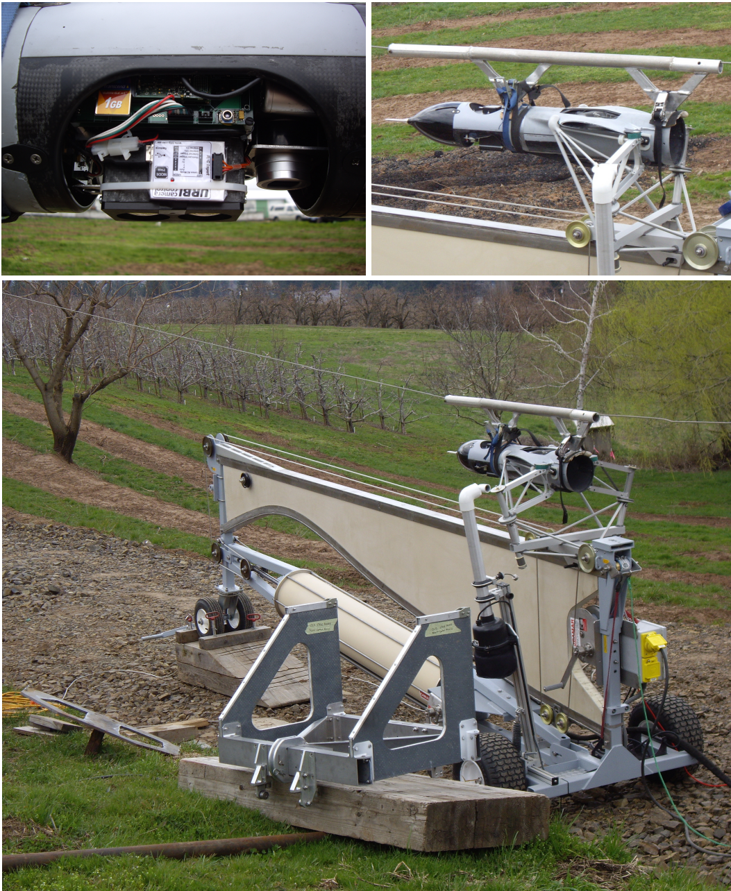
Figure G.1: The ScanEagle zip line testing setup and equipment. The ScanEagle CULPIS instrument package, shown on top left, is mounted in a mock ScanEagle fuselage and hung from a taught cable, shown on top right, and launched using a pneumatic catapult, shown in the bottom figure.
