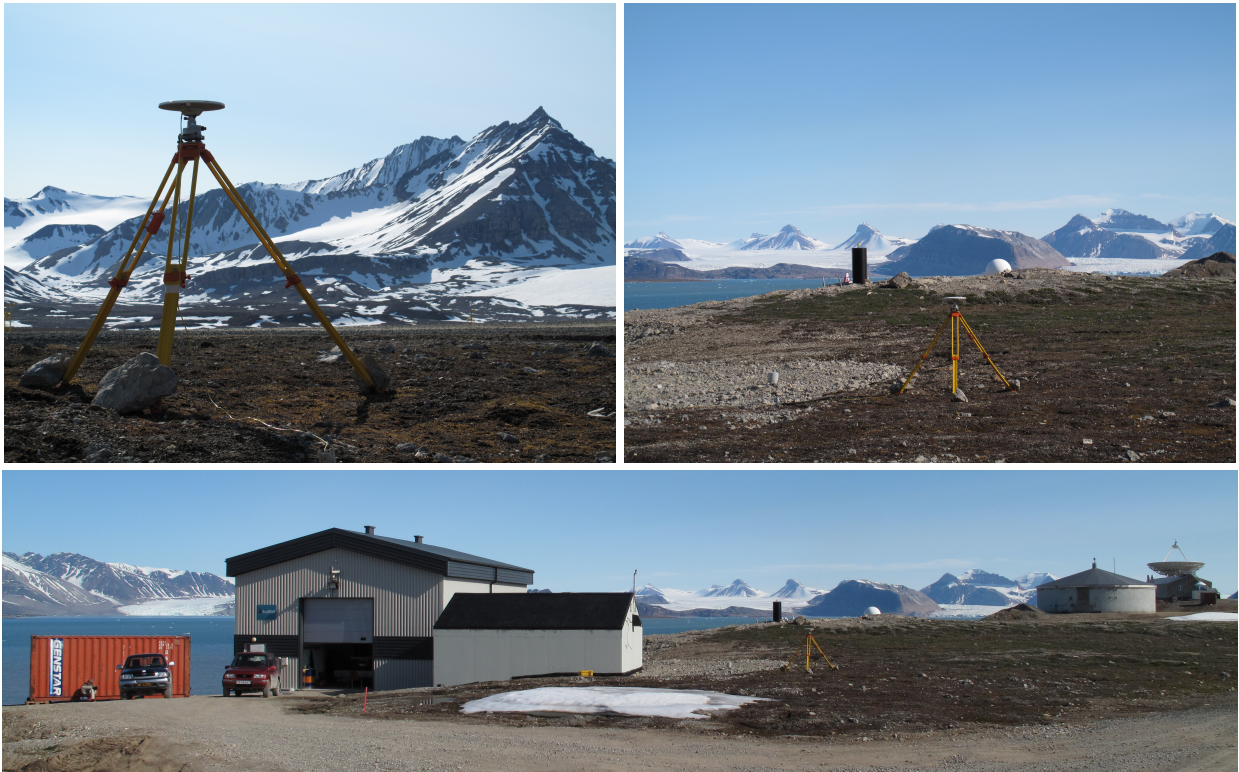
Figure H.1: The CASIE NYCU temporary GPS reference station environmental surroundings. The GPS station was located in the vicinity of large mountains, several buildings, and a gravel roadway that saw limited traffic.
