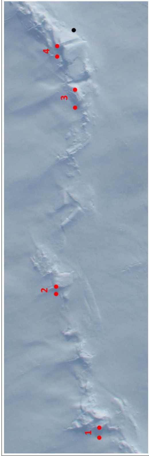
Figure M.1: Sea ice ridge heights calculated from the length of shadows in a photograph collected during CASIE. This ridge is part of the same ridge complex presented in Figure 6.2 on page 100. The ridge height calculation is described by Equation M.1. This image was collected from 200 m AGL at 15:26:43 UTC, and is located at 80°17'6" N, 4°27'57" E. Based on this time and location, the solar elevation angle, \theta , was determined to be 24.98°. The numbered ridge features were found to have the following heights: (1) 1.01 m, (2) 0.69 m, (3) 1.57 m, (4) 1.06 m. The black dot is located at a point that appears to represent the nominal ice surface elevation.
