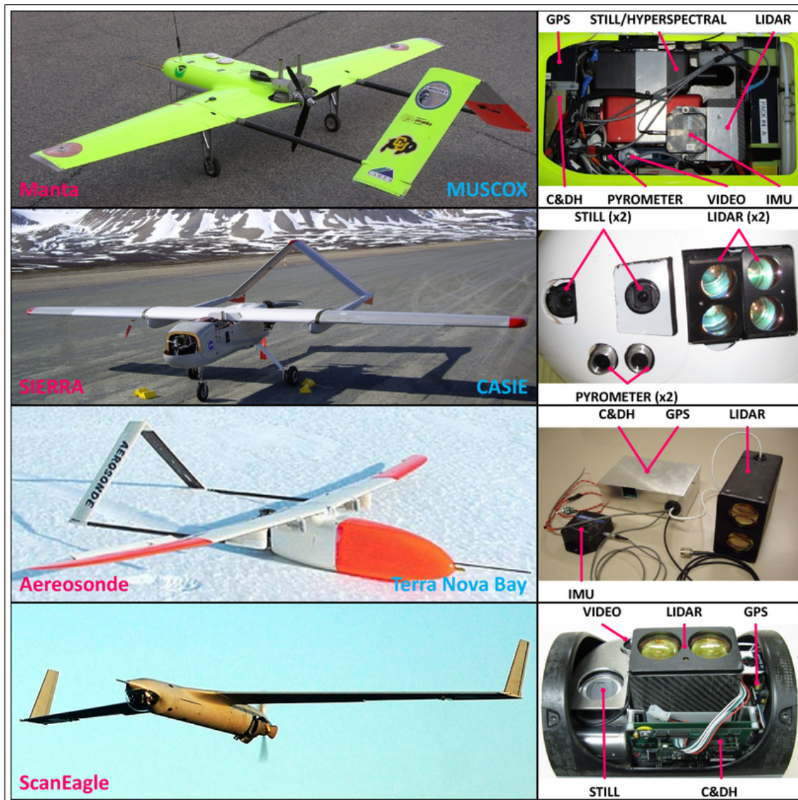
Figure 3.1: The UAS in which the CULPIS has been integrated (left panels) and their associated payloads (right panels). The campaigns in which they have been involved are listed in blue. Some of the CULPIS components and ancillary sensors are not visible within the images.
